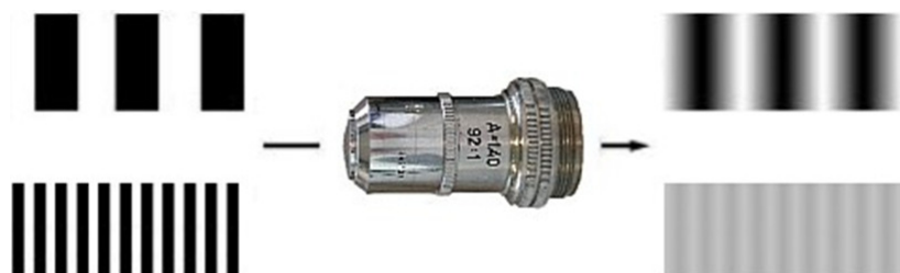
Figure 1. Resulting image from a line pattern, as seen through a microscope objective. Image contrast decreases to zero when line spacing reaches the theoretical limit of resolution.
